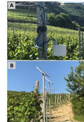
Picture 2: A) Device transmitting VS along the vibrational vineyard set in northern Italy to control grapevine leafhoppers; B) Solar panels providing energy to the vibrational devices. Credit: Fondazione Edmund Mach and Biogard® (Italy).
