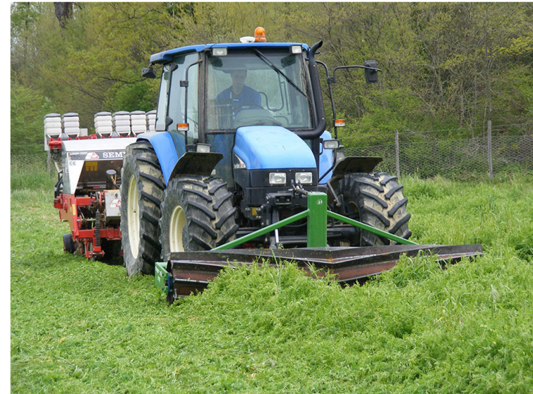
Fig. 1. Roller crimper (chevron design Rodale-type built by the farmer) mounted on the front of the tractor and coupled with a rear-mounted direct drill machine (Semeato SPE 06), carrying out hairy vetch (cv. Haymaker Plus) termination and sunflower (hybrid LG 55-57 HO) no-till sowing in one pass. Picture taken by Daniele Antichi at the farm hosting the trial (Tuscany, Italy) the 19th March 2014.
