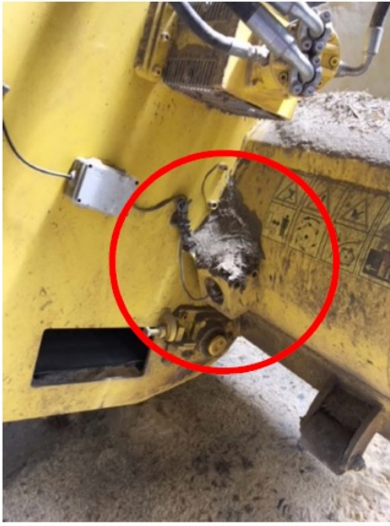
Fig. 1. The microwave moisture sensor positioned behind the loading drum of the TMR mixer wagon.
